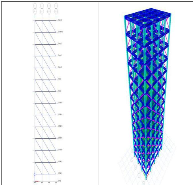
**Fig-3:** Elevation and 3D view of RC frame structure with diagonal bracing
